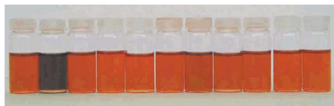
Figure 2. Colour changes induced on L^1 ( 1 \times 10^{-3} mol dm^{-3} ) in DMSO: from left to right: no anion, fluoride, chloride, bromide, iodide, hydrogenosulfate, dihydrogenophosphate, acetate, benzoate, cyanide and nitrate. A similar colour change in the presence of anions was found for this ligand in CH_3CN .
